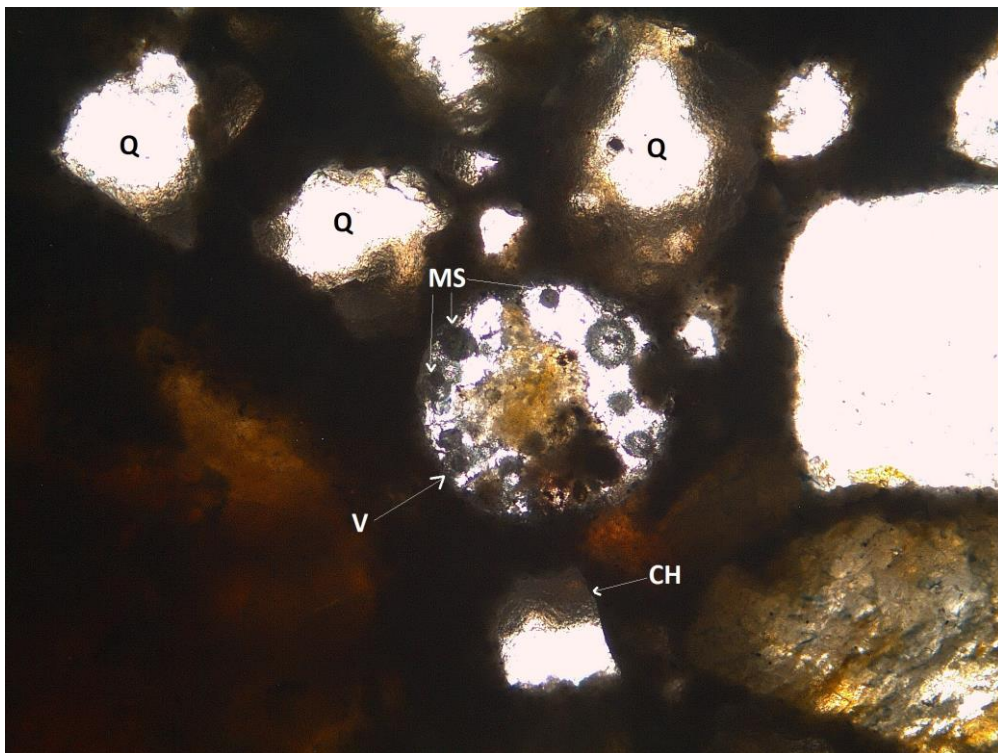
Figure 6.18 (b) Photomicrograph showing coating of calcium hydroxide ('CH') gel around periphery of medium size quartz ('Q') grains. Large size void ('V') was partially infilled with hydrated cementitious paste and undispersed microsilica ('MS') particles. [O.L. \times 5x ]
