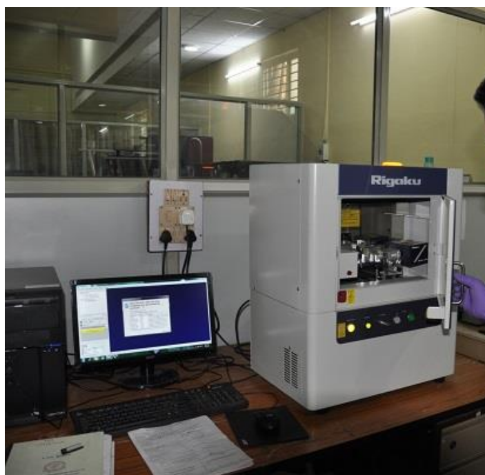
Figure 2.4 Experimental setup of X-ray diffractometer, CIF-IIT (BHU), (Rigaku Miniflex II, Japan).
