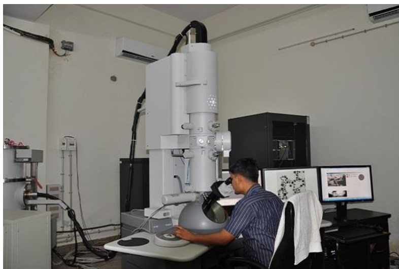
Figure 2.8 Experimental setup of TEM measurement, CIF-IIT (BHU), (FEI Tecnai G2 20 TWIN, USA).
