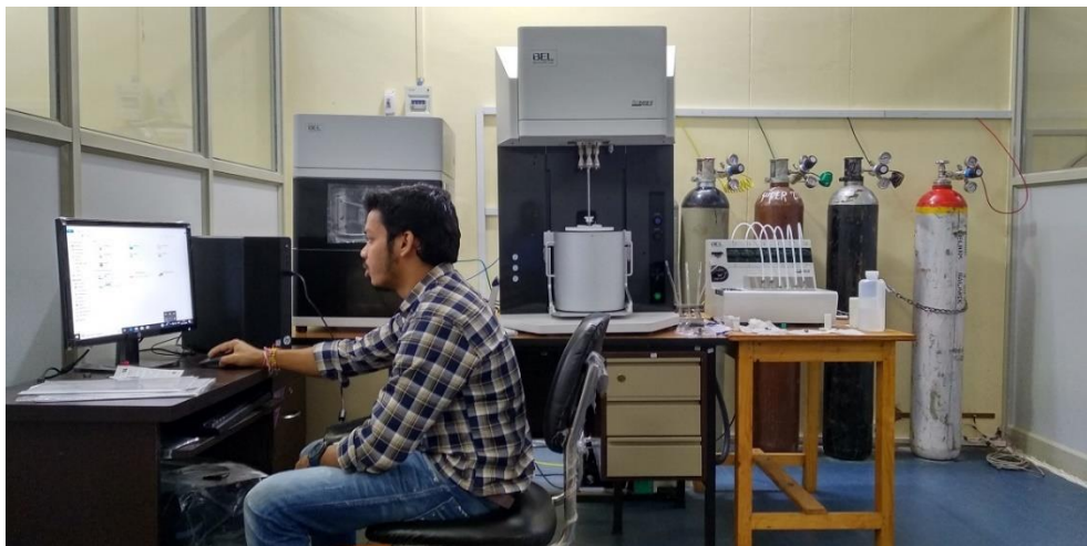
Figure 2.15 BET surface area measurement setup, CIF-IIT (BHU), (MicrotracBEL BET instrument).
