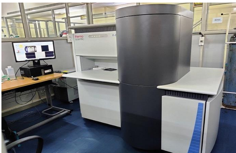
Figure 2.10 Experimental setup of XPS spectroscopy, CIF-IIT (BHU), (Thermo Fisher Scientific's K-Alpha spectrometer).
