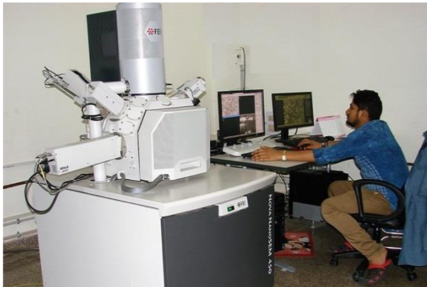
Figure 2.6 Experimental setup of SEM measurement, CIF-IIT (BHU), (Nova Nano SEM 450).
