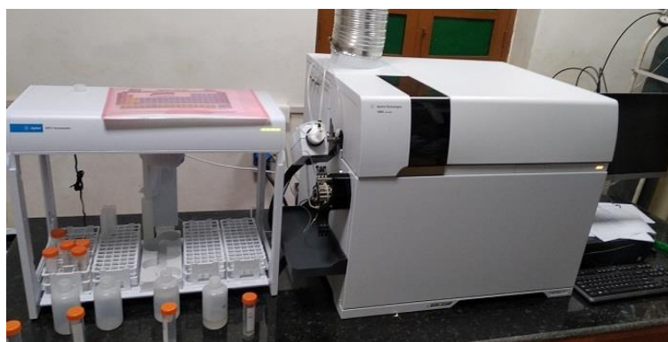
Figure 2.12 Experimental setup of ICP-MS, CIF-IIT (BHU), (Agilent 7800 ICP-MS mainframe).
