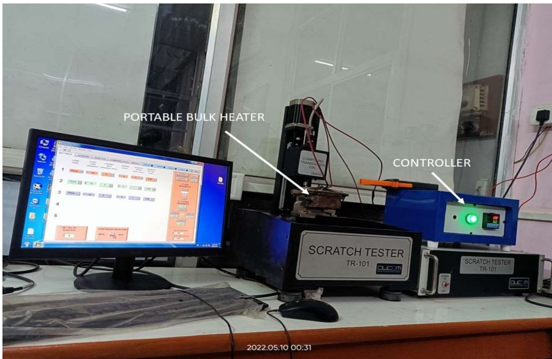
Figure 3.20: Schematic of using the portable bulk heater on scratch tester
