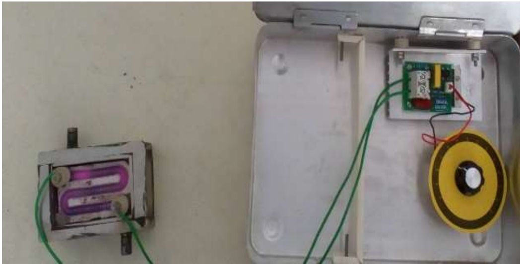
Figure 3.15: Heat controller with insight of setup
