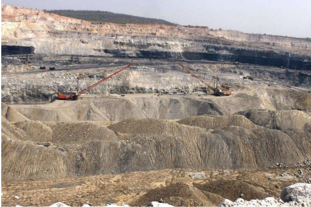
Figure 5.5: Dragline working in horizontal tandem at Nighai project.
