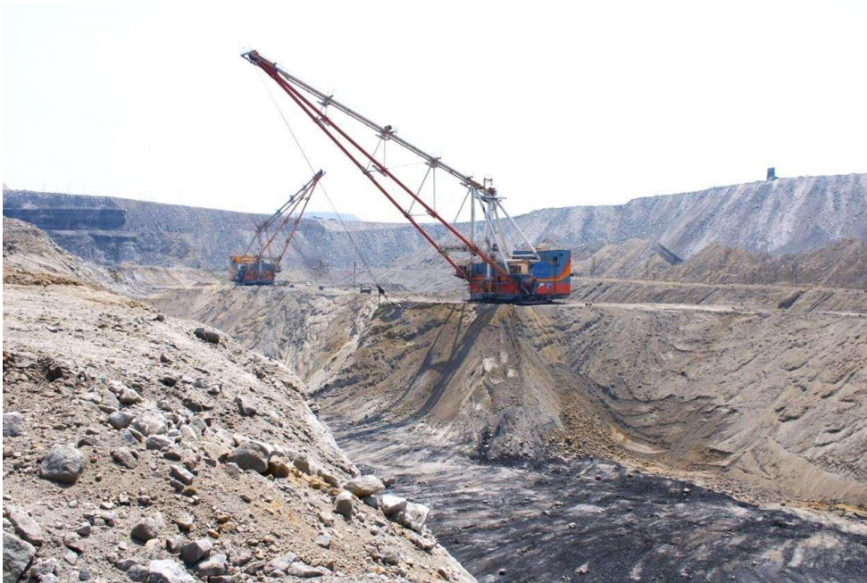
Figure 5.7: Dragline working in horizontal tandem at Dhudhichua project.
