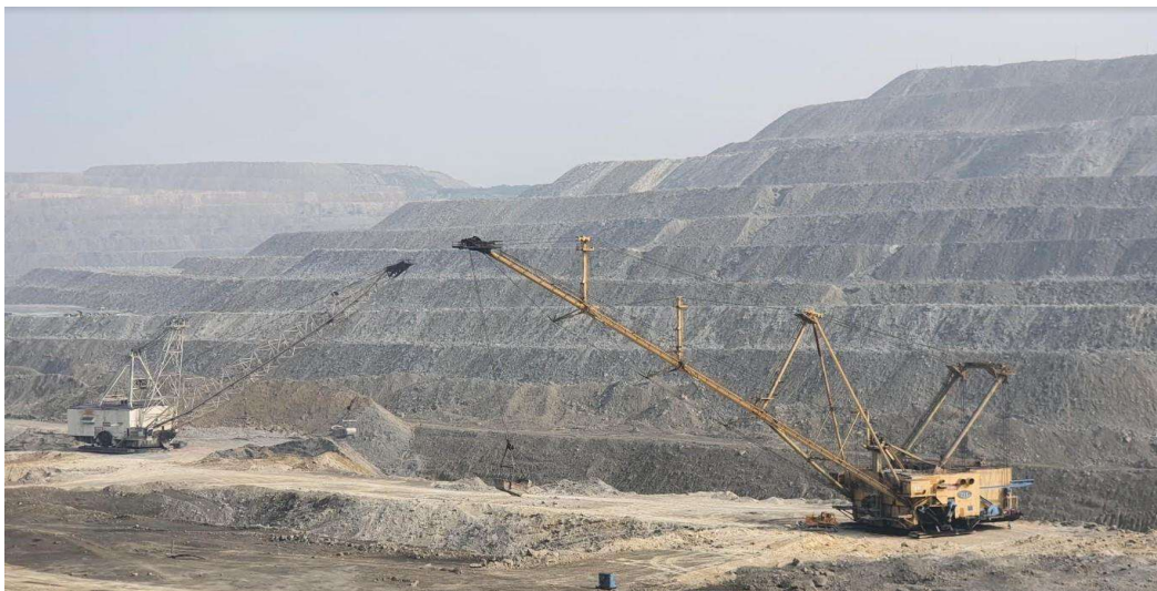
Figure 5.10: Dragline working in horizontal tandem at Jayant project.
