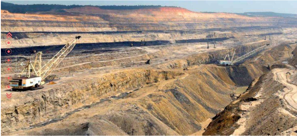
Figure 5.8: Dragline working in vertical tandem at Bina project.
