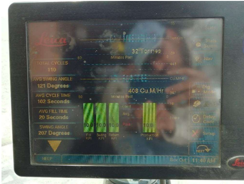
Figure 5.14: Leica dragline monitoring system showing cycle time and swing angle information.
