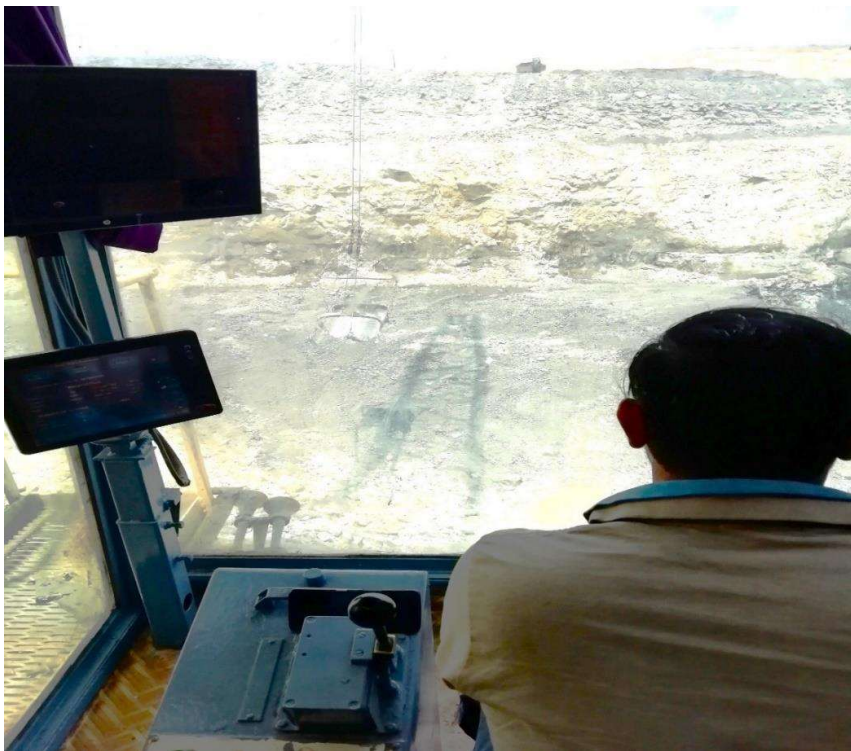
Figure 5.11: Leica on-board monitoring system of a dragline model W-2000 at NCL mine.
