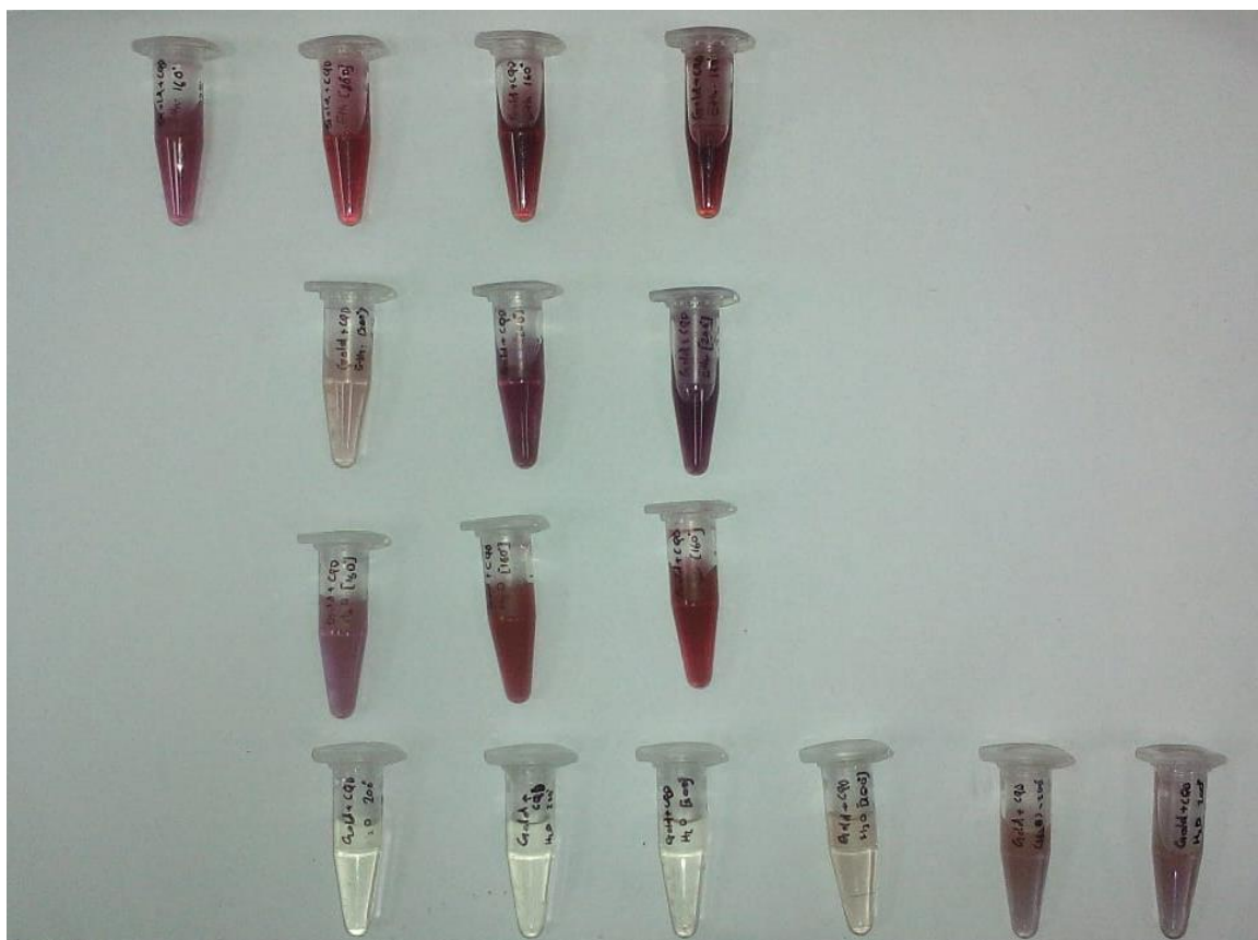
Figure 4.6: CQD concentration- dependent Synthesis of Gold Nanoparticles. The four rows represent the use of E160, E200, W160 and W200 respectively showing most spontaneous reaction with E160 and least with W200 using CQD concentrations 0.025-0.5 v/v
