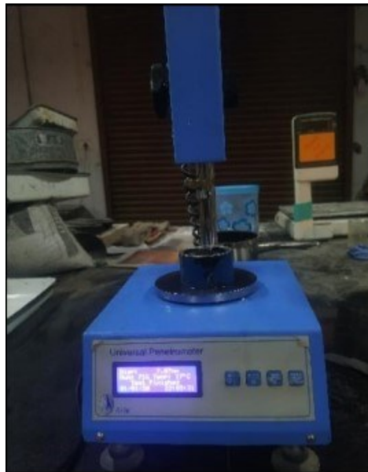
Figure 6-2 Penetration test setup
