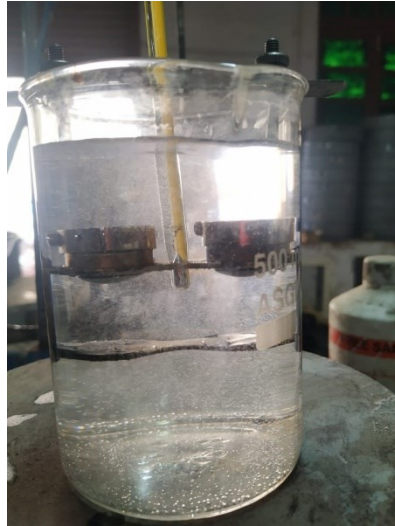
Figure 6-3 Test assembly for softening point test
