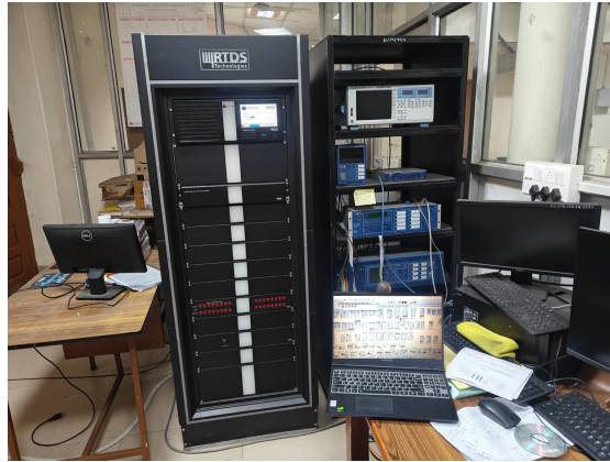
Figure 25: Image showing RTDS connected to Work Station
