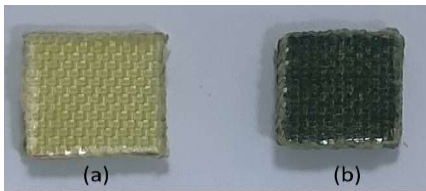
Figure 4.10 Thermal conductivity samples of (a) AF/Epoxy, (b) CAF-FCNT/Epoxy
