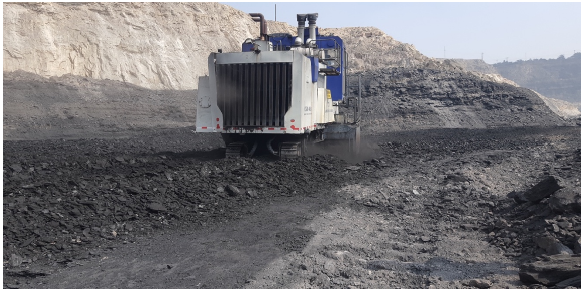
Figure 3.4: L&T made KSM403 operating in windrowing mode at NOCM
