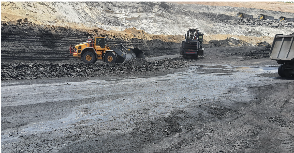
Figure 3.9: Wirtgen made 2200 SM 3.8 in conjunction with front-end payloaders at BOCM
