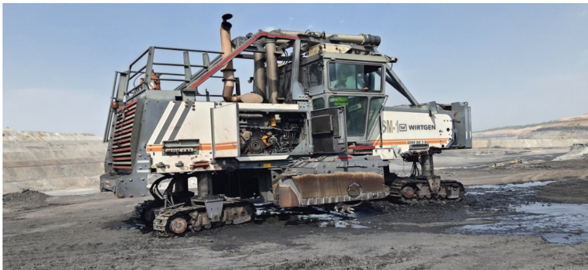
Figure 3.12: Wirtgen made 2200 SM 3.8 deployed at PEKB
