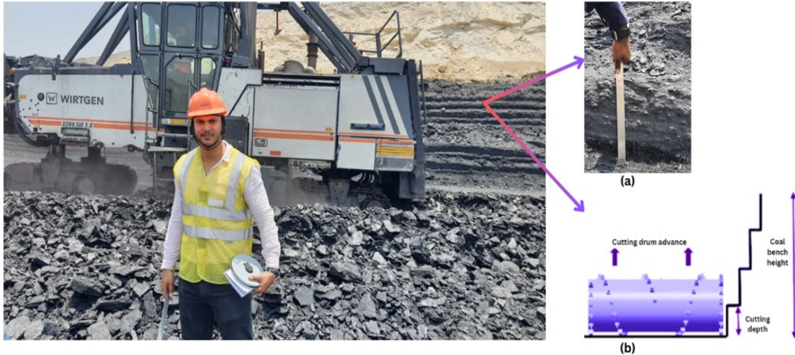
Figure 3.23: Measurement of SM cutting depth at BOCM: a) front view of coal bench slope; b) sectional view of coal bench
