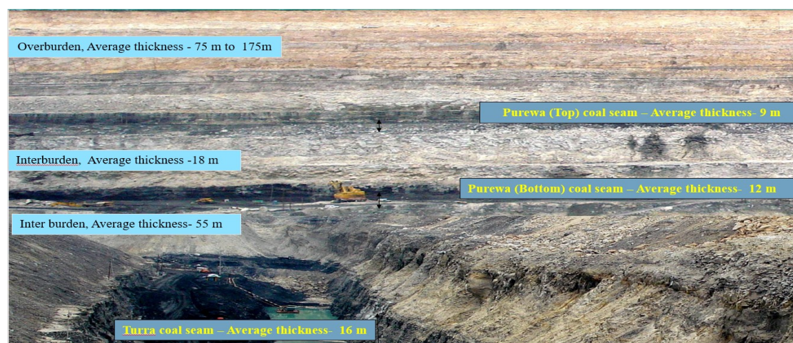
Figure 3.3: Cross-sectional view of Nigahi opencast coal mine
