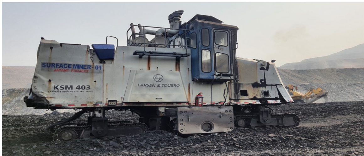
Figure 3.7: L&T made KSM403 operating in windrowing mode at JOCM
