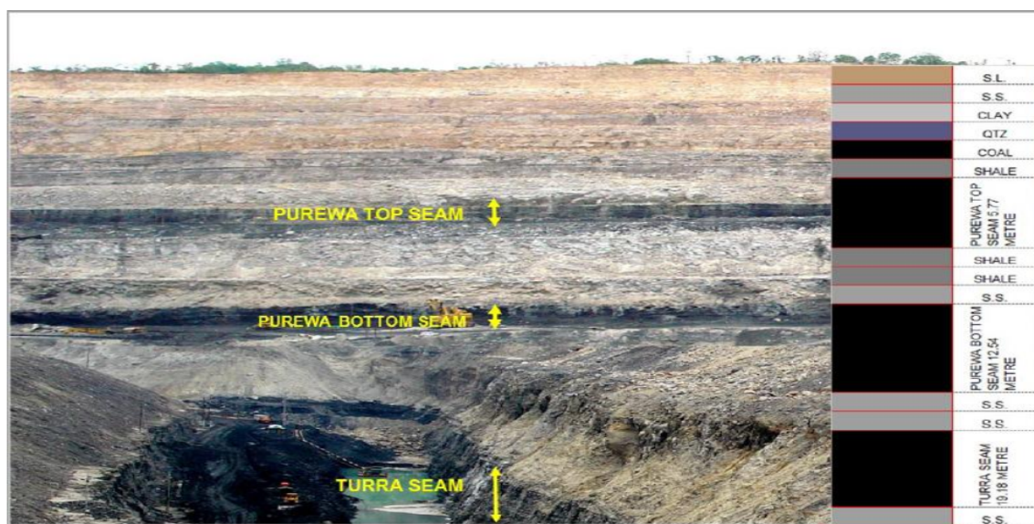
Figure 3.6: Cross-sectional view of Jayant opencast coal mine
