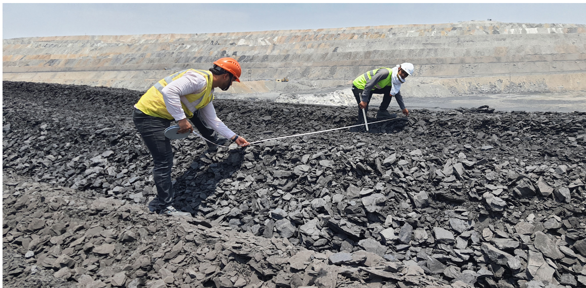
Figure 3.21: Measurement of center to center spacing between two adjacent cuts of SM
