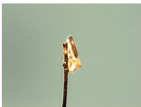
Figure 5.33. Crystal image of compound AK-2 during SC-XRD analysis.
