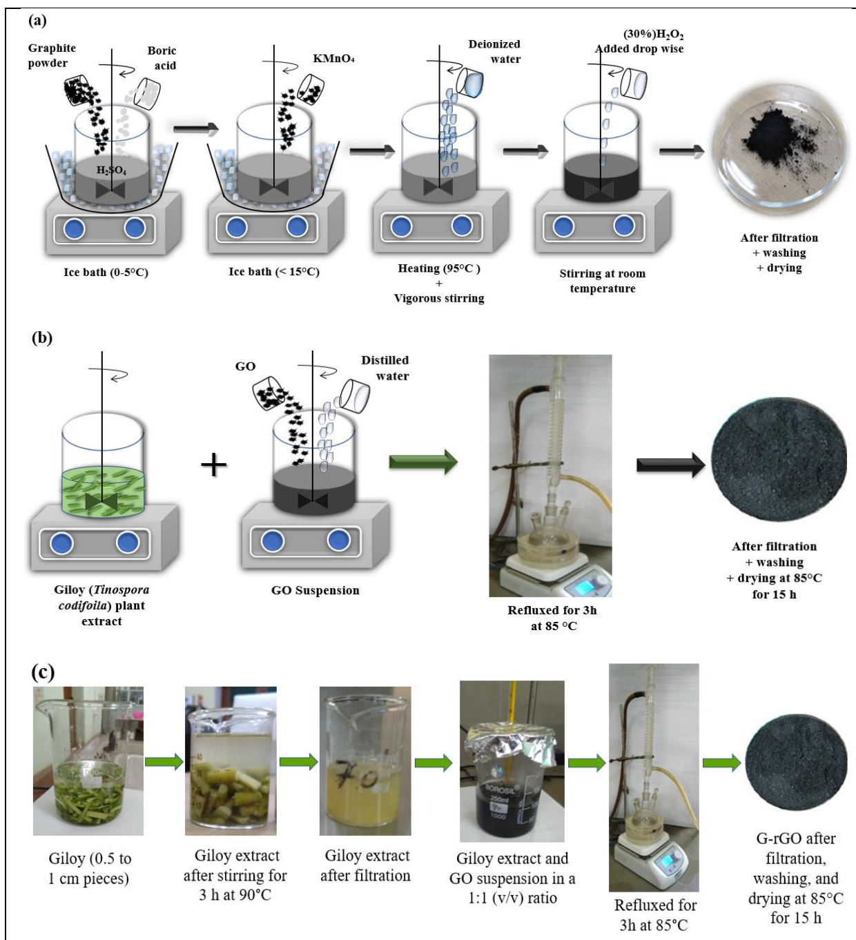
Fig. 4. 1 (a) A schematic illustration of the GO's using modified Hummer's method, (b) An illustration of the G-rGO from T. cordifolia , and (c) A typical presentation of green synthesis of G-rGO from T. cordifolia plant extract.
