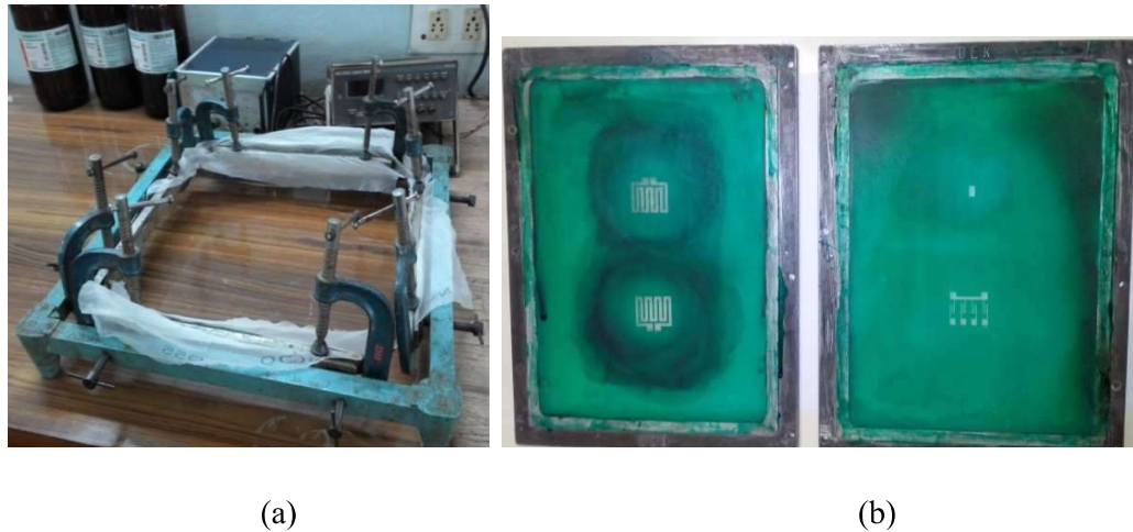
Fig. 2.14 (a) Manual screen preparation tool (b) Prepared screens
