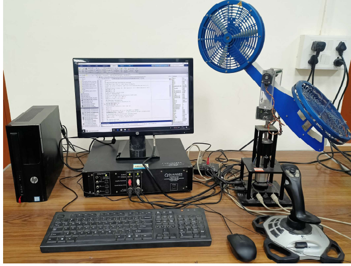
Figure 7.1: Experimental setup of two-DOF helicopter.
