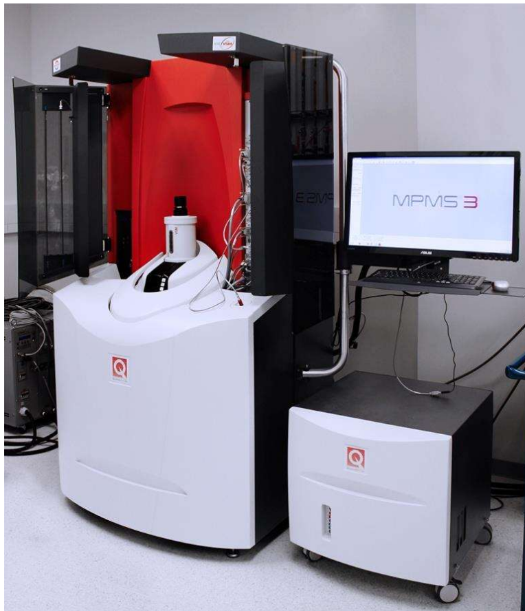
Figure 2.6 Superconducting quantum interference devices (SQUID) (Quantum Design, MPMS 3)
