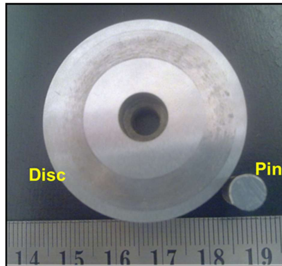
Figure 2. Pin-on-disc wear test set-up.
