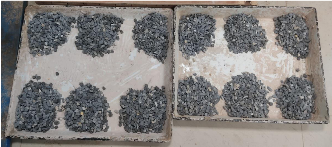
Fig. 3.21 Pictorial representation of tire chips - aggregates mixture for a group of 12 granular piles.
