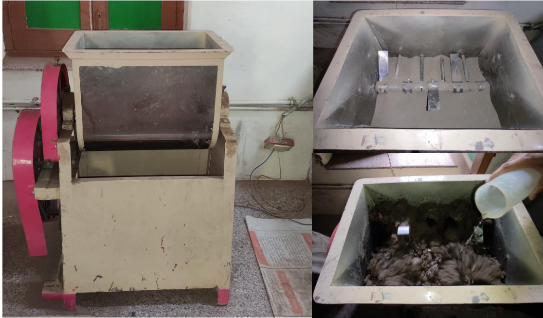
Fig. 3.11 Mechanical soil mixing machine for preparing soil paste.
