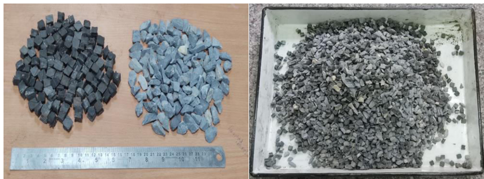
Fig. 3.4(b) Tire chips – aggregates mixture used in the present study.
