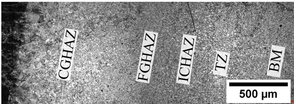
Figure 4.11: Optical micrograph of sample 09: Fusion Zone and Heat affected zone containing CGHAZ, FGHAZ, ICHAZ, TZ and BM
