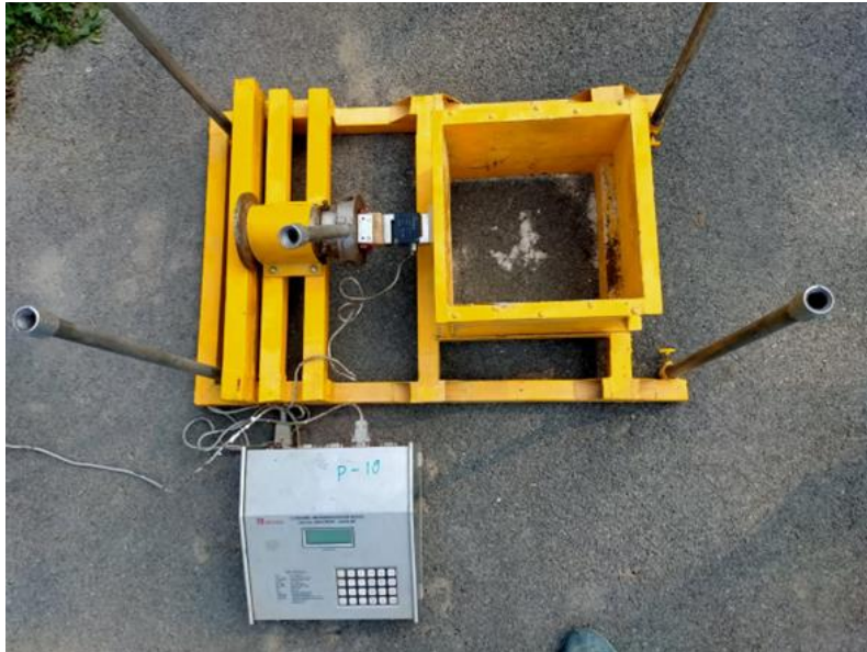
Figure 3. 3 Field Shear box with load cell and data logger
