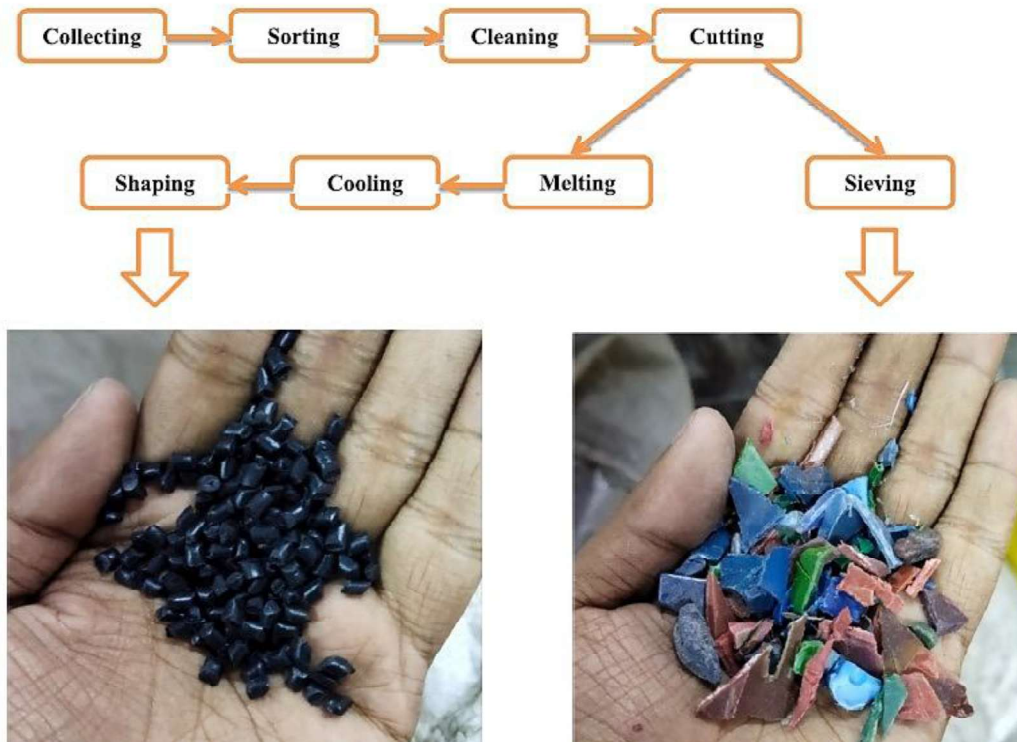
Fig. 2.15 Flowchart depicting the process of fine and coarse plastic aggregates (Saha et al. 2023)).
