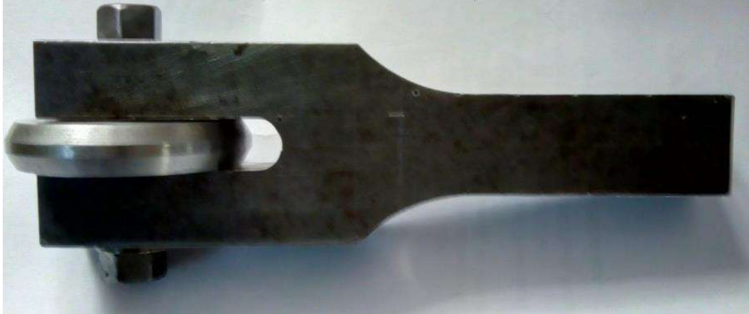
Figure 2.10: Roller assembly used for initial flow forming operation.
