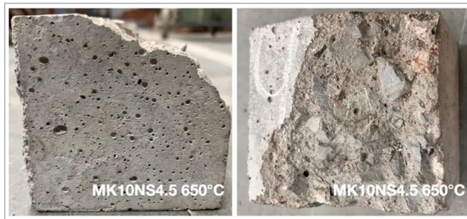
Figure 6.39 Spalled cube of MK10NS4.5 at 650°C
