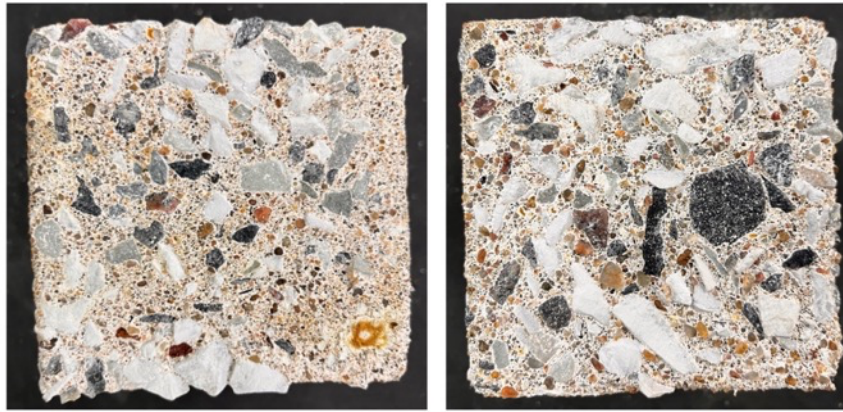
Figure 6.16 Concrete cubes after 28 days of sulfuric acid exposure
