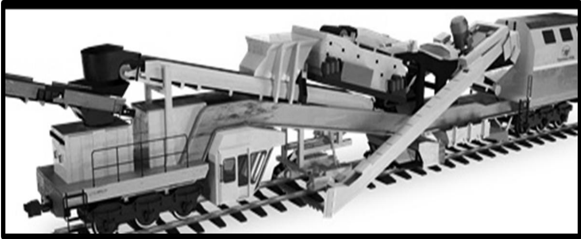
Fig.1.3: Schematic view of ballast cleaning machine
