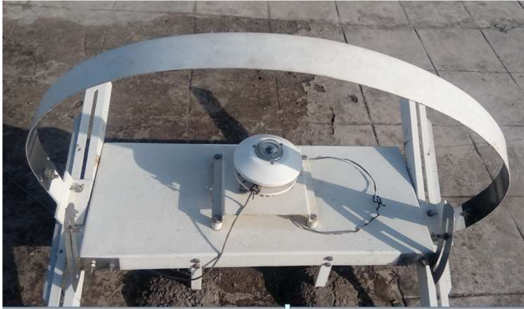
Figure 3.19: Photograph of pyranometer to measure diffuse radiation
