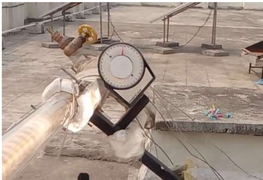
Figure 3.10: Photograph of circular magnetic needle to measure tilt angle of PTC
