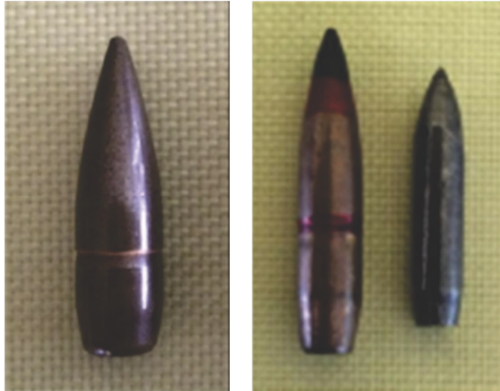
Fig. 1.2: 7.62mm small arms ammunitions (a) ball ammunition and (b) AP ammunition with its hard steel core(Crouch, 2016).
