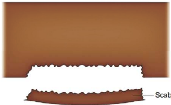
Fig 1.8 : Schematic of spalling process(Crouch, 2016).
