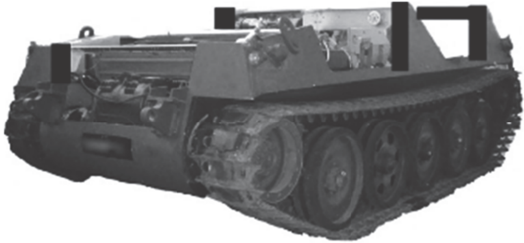
Fig. 1.15: The exposed hull of Warrior tracked vehicle showing the use of AA 7017 plates in its hull portion (Hazell, 2015).
