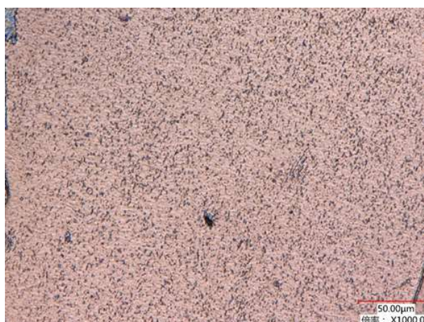
Fig. 4.10 Optical image of CVD-grown graphene for 10 min reaction time at 850 °C under an acetylene flow rate of 6 sccm.
