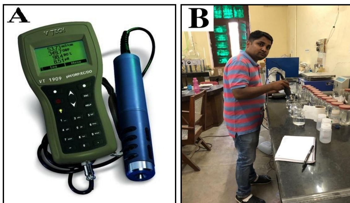
Figure 4.8 Photograph showing (A) Multi-parameter (B) Analysis of water samples using multi-parameter kit
