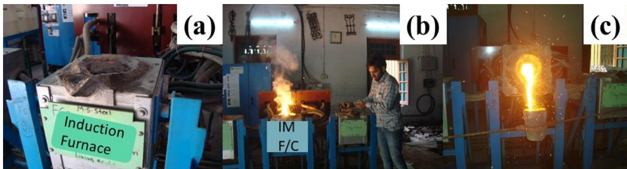
Figure-6.9 Photographs of furnace used to melting studies: a) Isometric view; b) Cold Charging, Melting & Sampling; c) Pouring into crucible
