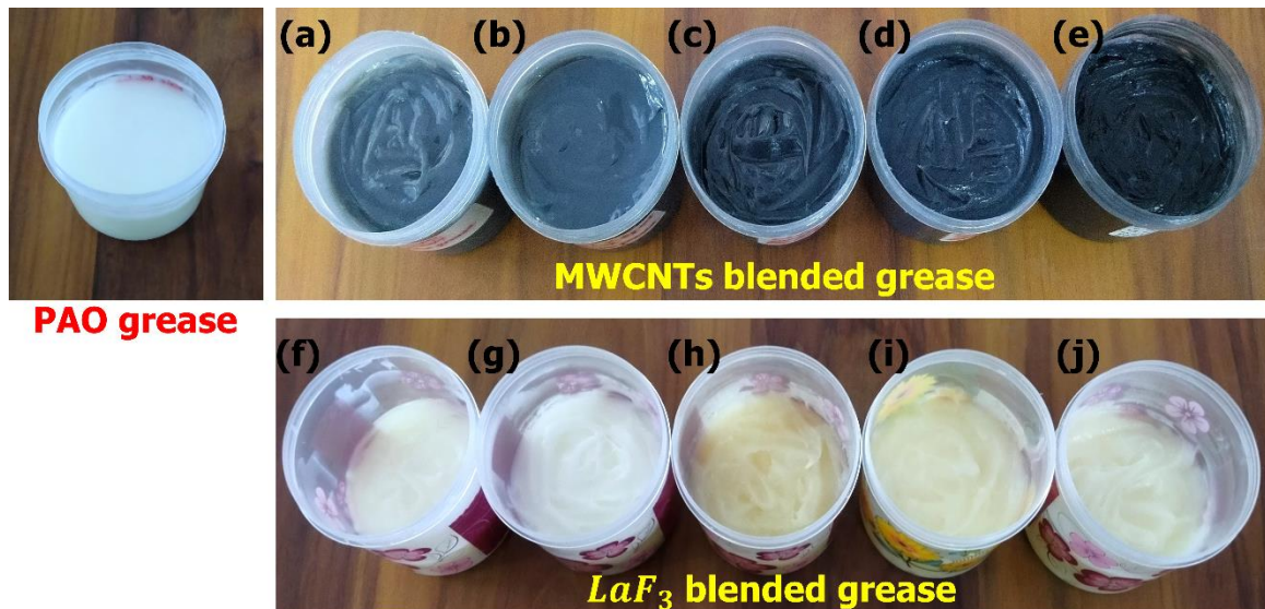
Figure 7.1: PAO 100 grease having a variable concentration of MWCNTs and LaF 3 : (a, f) 0.025 wt.%, (b, g) 0.05 wt.%, (c, h) 0.075 wt.%, (d, i) 0.1 wt.%, and (e, j) 0.15 wt.%
