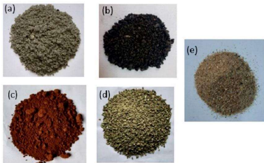
Figure 3.3: Material used for mold preparation (a) blast furnace slag (b) ferrochrome slag (c) red mud (d) olivine sand (e) silica sand
