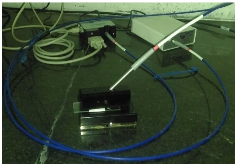
Figure 3.7 UV– Vis Diffuse Reflectance Spectrophotometer
