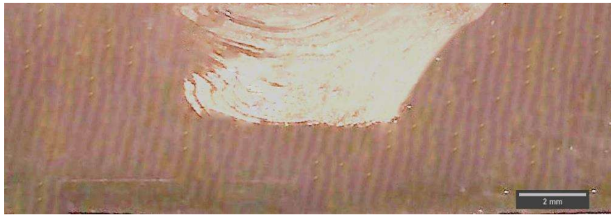
Figure 5. 2 The cross-sectional macrostructure of FSPed Cu/FA surface composite
