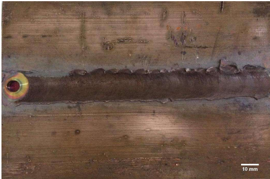
Figure 5. 1 The surface appearance of FSPed Cu/FA surface composite
