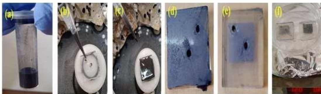
Fig.17: Preparation of graphene cathode: Picture of (a) graphene solution, (b), (c)& (d) coating of graphene solution on FTO using the spin coating method, (e) graphene coated substrate, (f) heating of graphene cathode.
