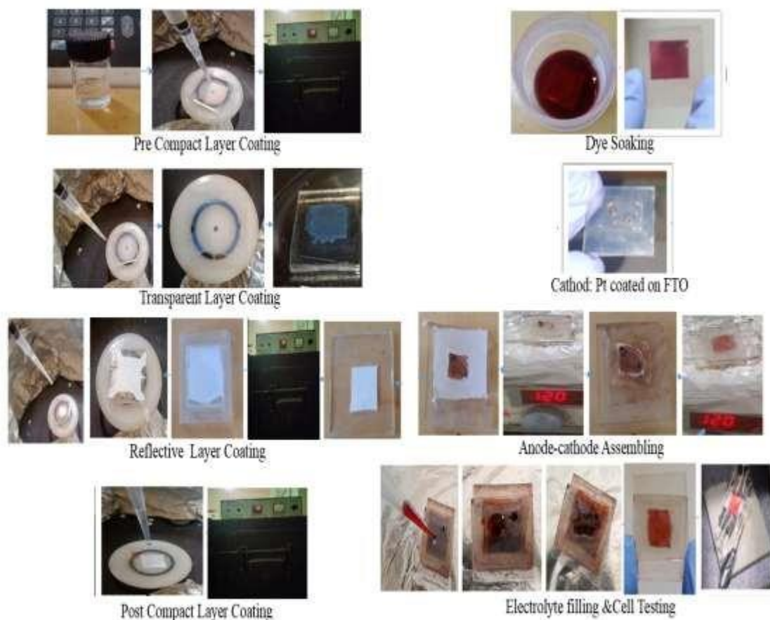
Fig.7: Fabrication steps of DSSC i.e. images of steps of pre-compact layer coating, transparent layer coating, reflective layer coating, post compact layer coating, dye soaking, Pt coating on CE, anode-cathode assembling and Electrolyte filling & Cell testing.
