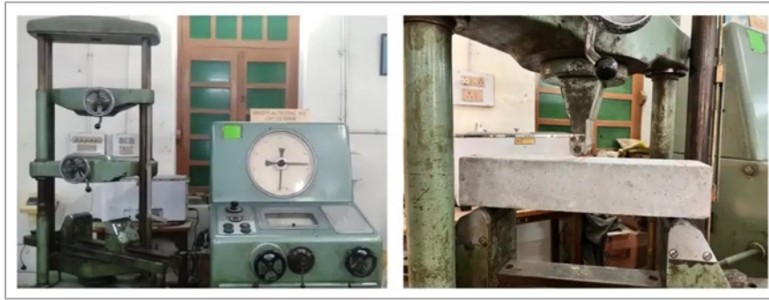
Figure 5.6 Flexural strength test of concrete prism on the universal testing machine. (Dept. of Civil Engineering, IIT BHU)
