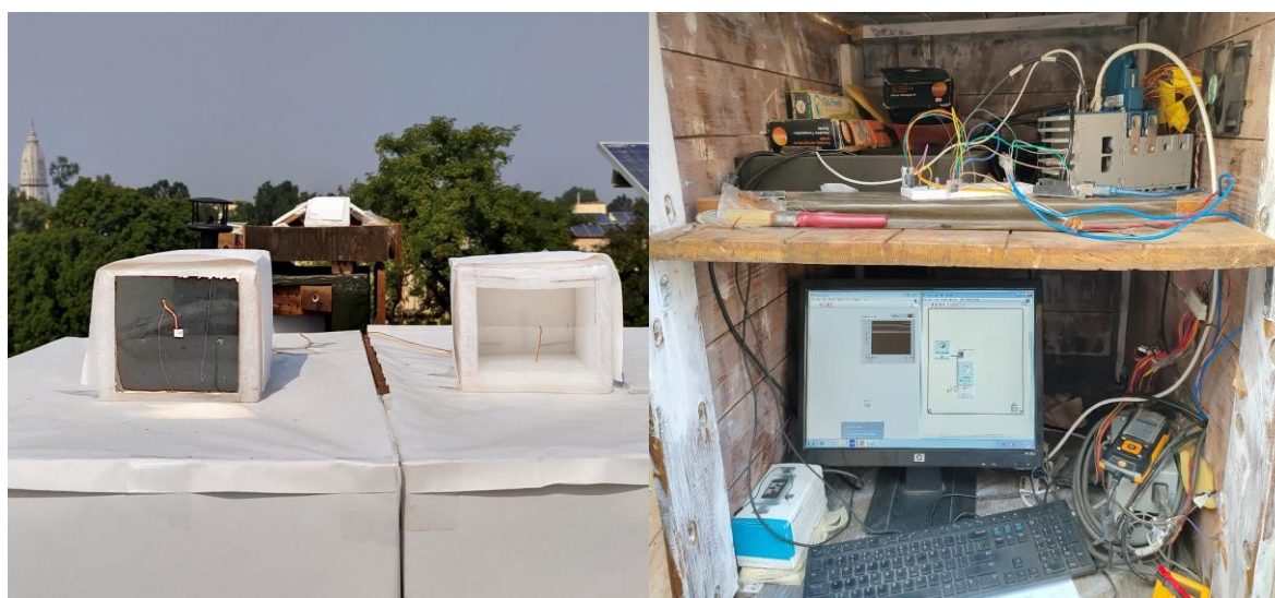
Figure 4.22 Experimental set-up under sunlight outdoor experiment.
