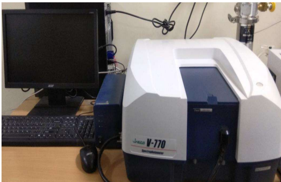
Figure 2.11: Experimental setup of JASCO V-770 UV-Vis spectrometer.
