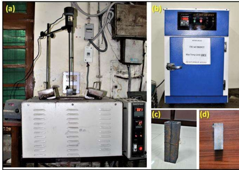
Fig. 2.1 (a) Stir-casting set up (b) Electric oven (c) Copper mould (d) As cast sample
