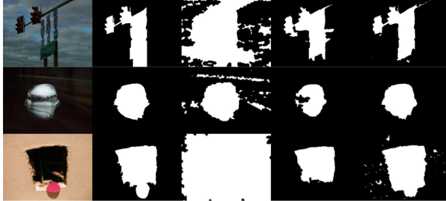
FIGURE 3.20: Comparing the results of salient object detection using only GVF, only MDC, and the proposed algorithm. First column: Original image; Second column: Ground truth; Third column: Output of using only GVF algorithm; Fourth column: Output of using only MDC saliency map; Final column: Output of the proposed algorithm.
