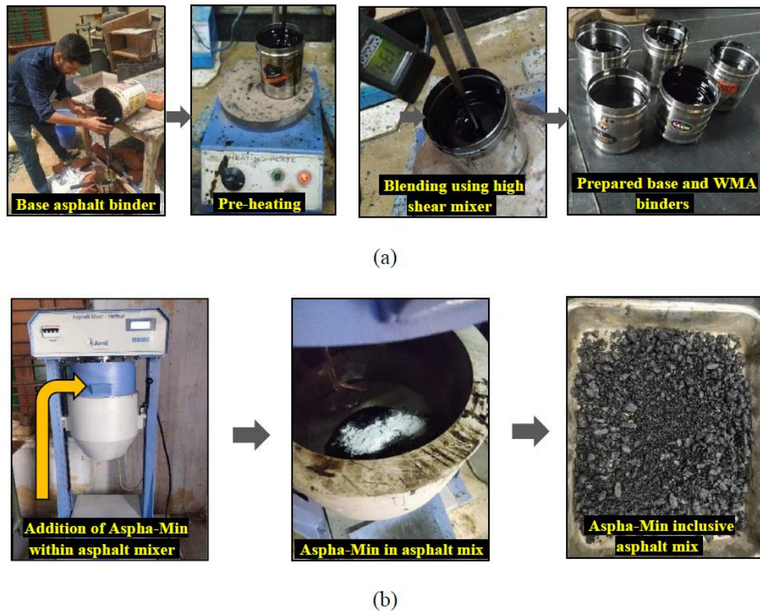
Figure 3.2. Stepwise preparation of WMA binder and mixtures (a) organic and chemical-based WMA binders and (b) foaming-based WMA mixture
