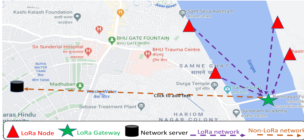
Figure 5.1: Illustration of a river water pollution monitoring using LoRa network in IoT.
