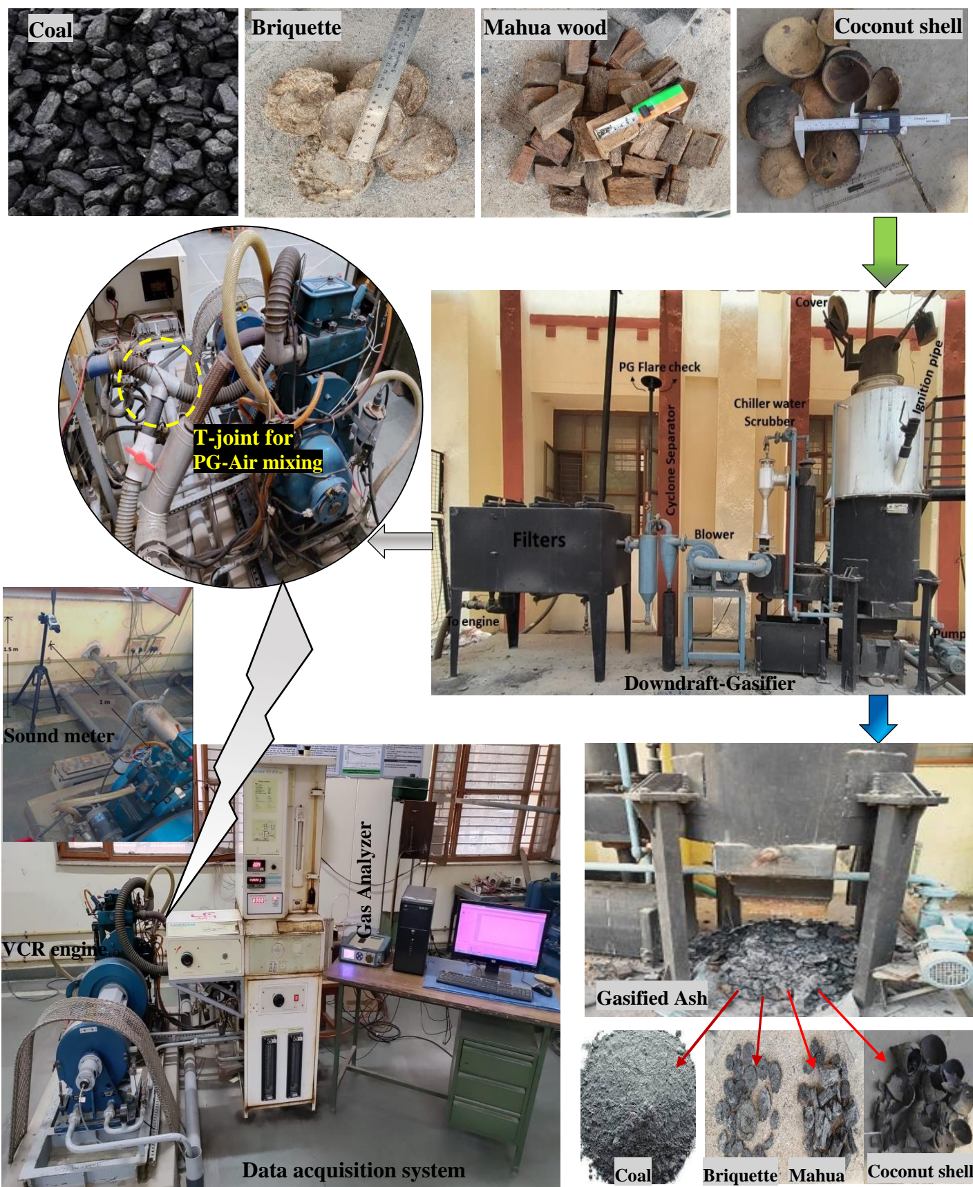
Figure 3.1.5. Experimental setup of downdraft gasifier integrated CI engine
