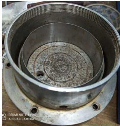
(e) Metal consolidation cell with collar
