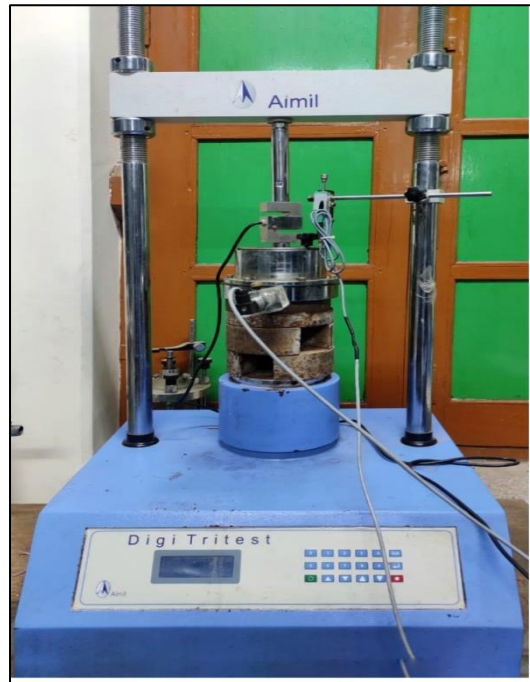
Figure 4.3 CRS and EKCRS loading assembly
