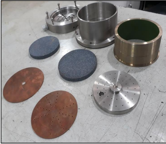
(c) Individual components of EKCL Oedometer
