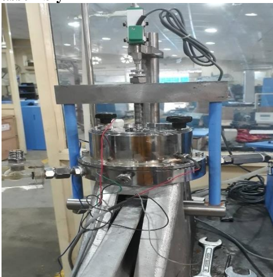
(a) Assembly EKCL Oedometer
