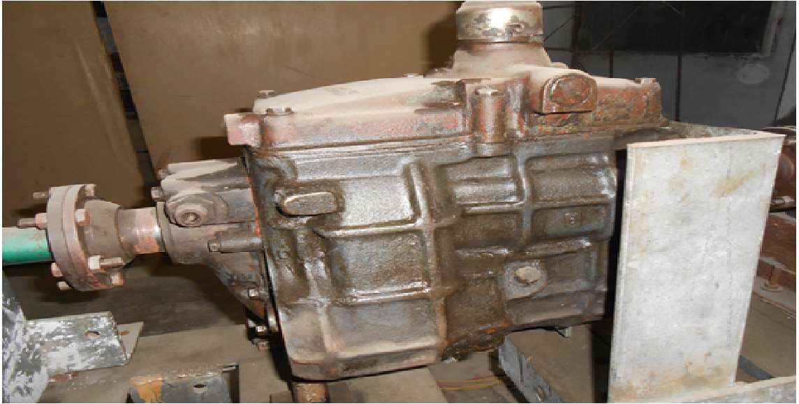
Figure 4.11: Additional gearbox incorporated for modification of 8 mm feedstock Continuous Extrusion setup
