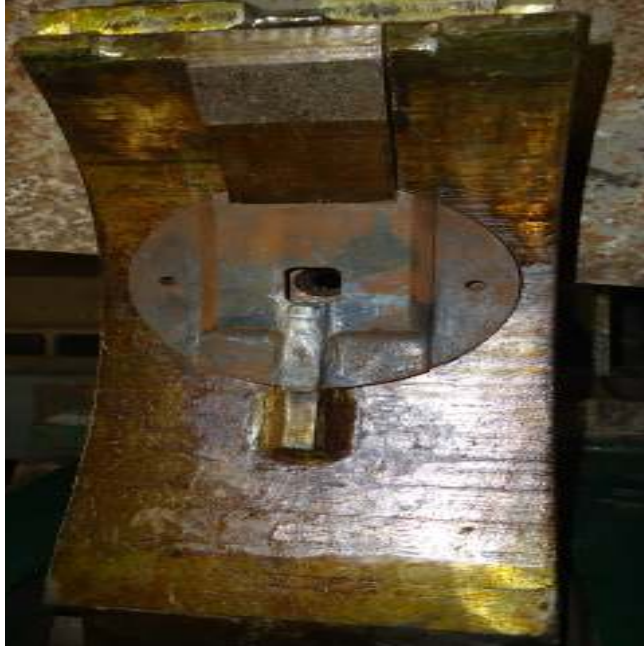
Figure 4.19: Extrusion Shoe for 9.5 mm feedstock Continuous Extrusion setup
