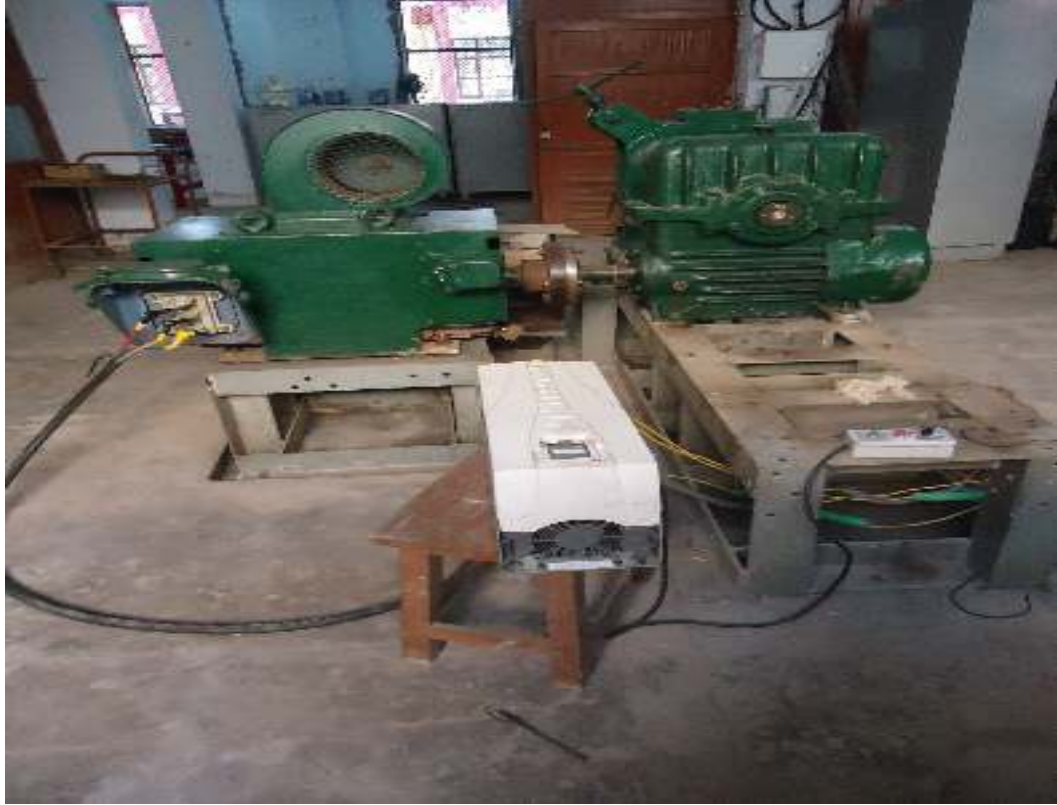
Figure 4.25: Design Developed and Fabricated Continuous Extrusion setup for 9.5 mm feedstock material
