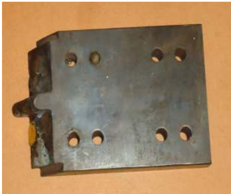
Figure 4.22: Scraper for 9.5 mm feedstock Continuous Extrusion setup
