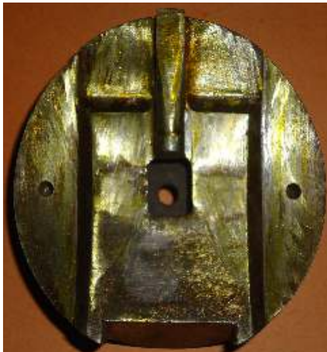
Figure 4.20: Abutment Die Chamber for 9.5 mm feedstock Continuous Extrusion setup
