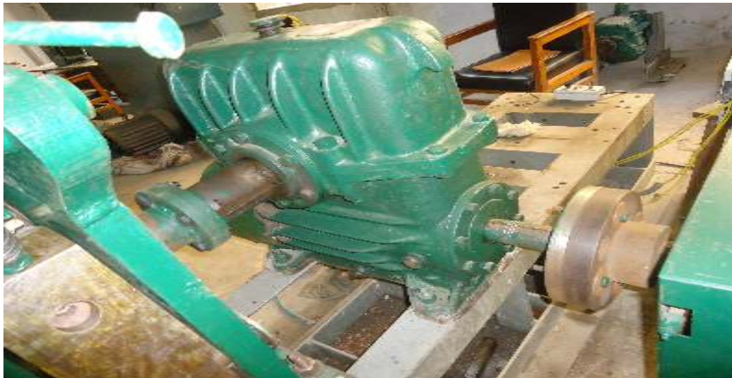
Figure 4.26: Close view of Design Developed and Fabricated Continuous Extrusion setup for 9.5 mm feedstock material
