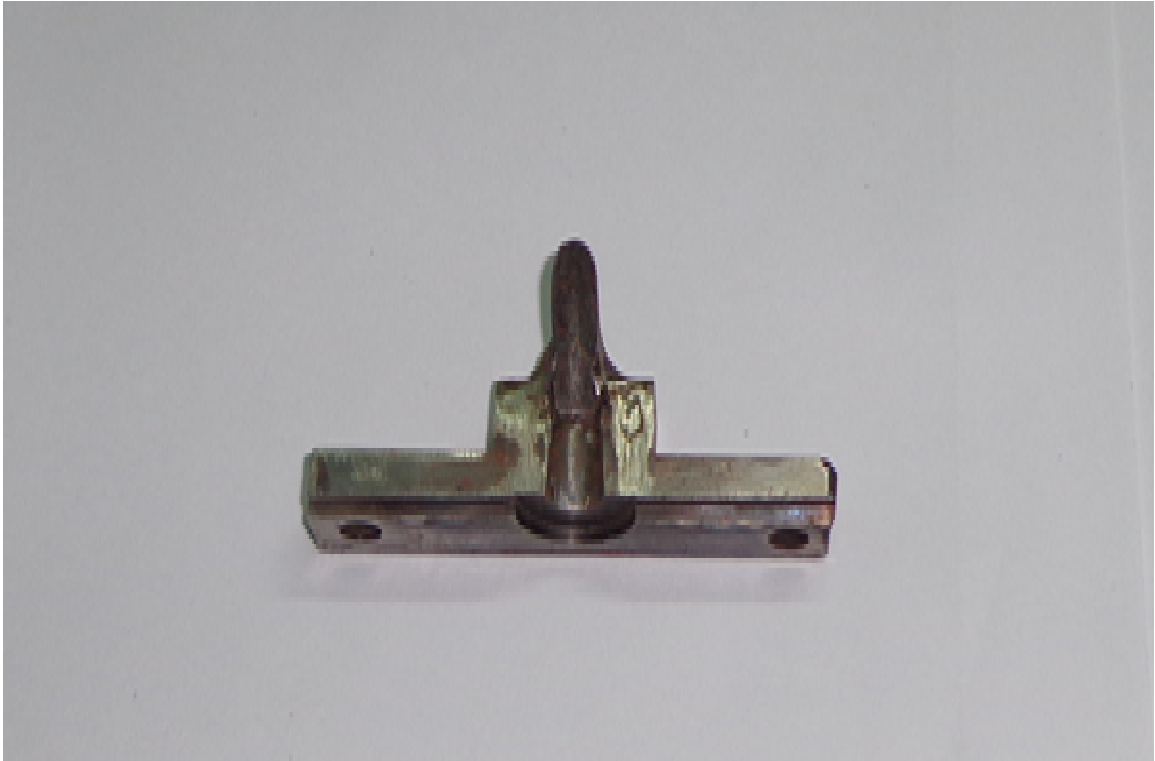
Figure 4.13: Modified abutment for 8 mm feedstock Continuous Extrusion setup
