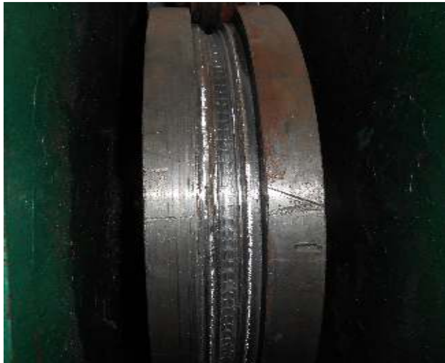
Figure 4.6 : Extrusion Wheel with circular groove for 8 mm feedstock material
