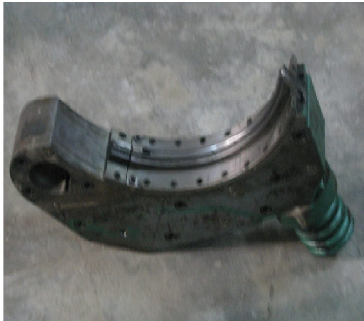
Figure 4.8: Grooved Extrusion shoe for 8 mm feedstock material
