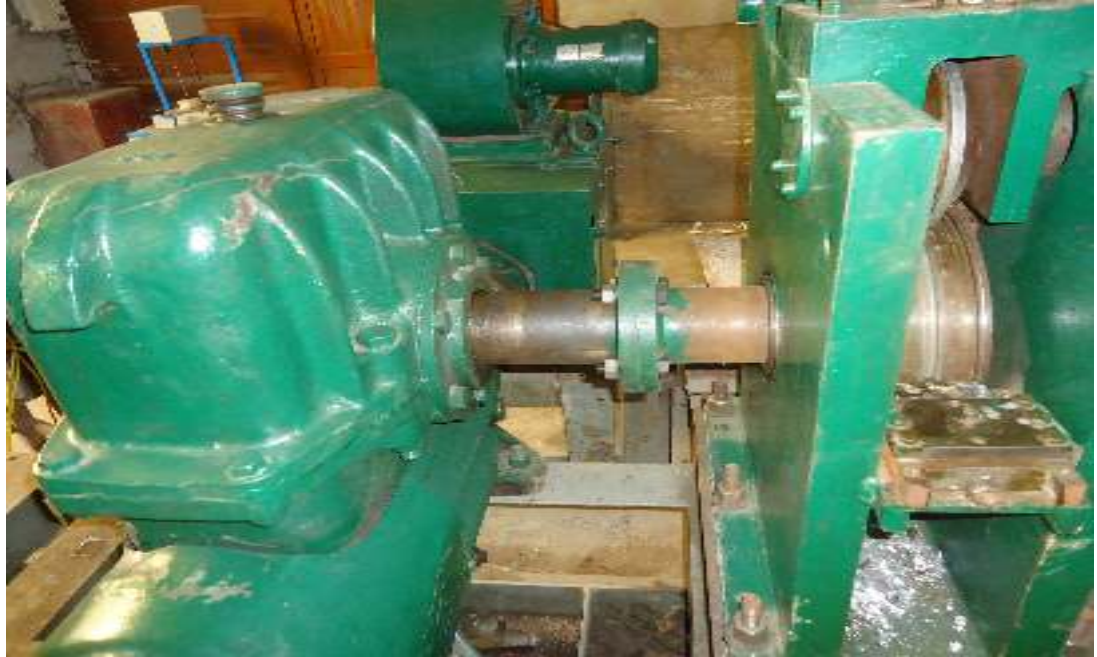
Figure 4.27: View of Gearbox coupled with Continuous Extrusion setup for 9.5 mm feedstock material
