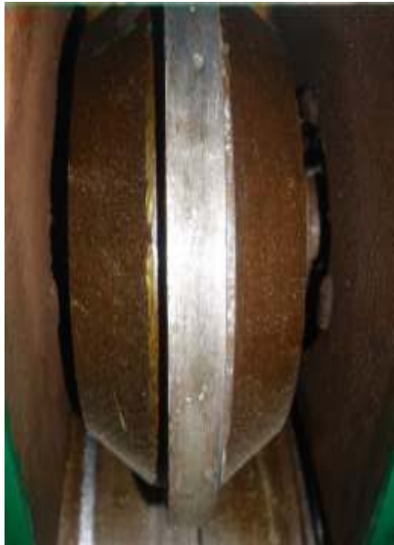
Figure 4.18: Coining Wheel for 9.5 mm feedstock Continuous Extrusion setup
