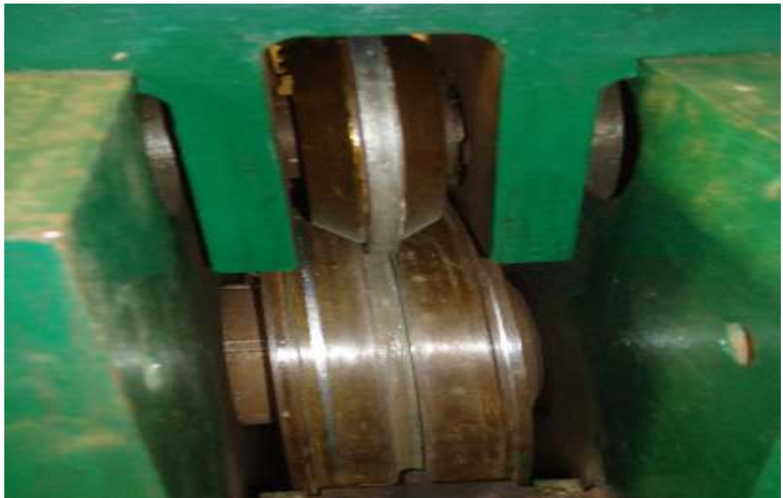
Figure 4.28: Close view of Extrusion Wheel, Coining Wheel and Scraper of Continuous Extrusion setup for 9.5 mm feedstock material
