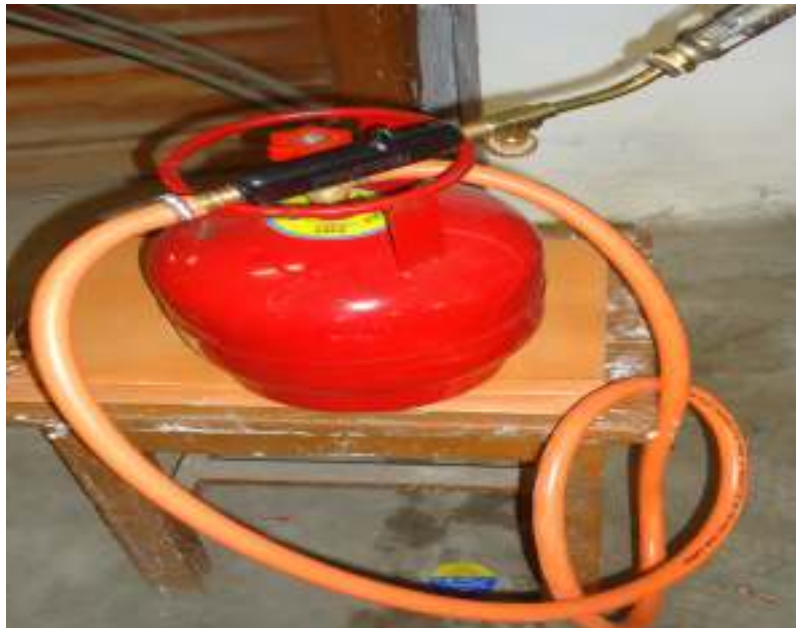
Figure 4.24: Die Chamber heating arrangement device for 9.5 mm feedstock Continuous Extrusion setup
