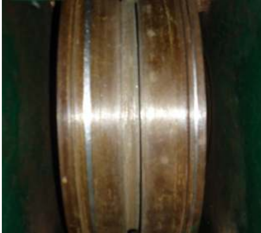
Figure 4.17: Extrusion Wheel for 9.5 mm feedstock Continuous Extrusion setup
