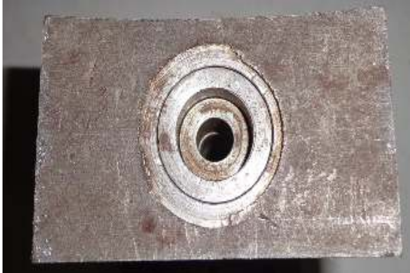
Figure 4.9: Extrusion die block for 8 mm feedstock Continuous Extrusion setup
