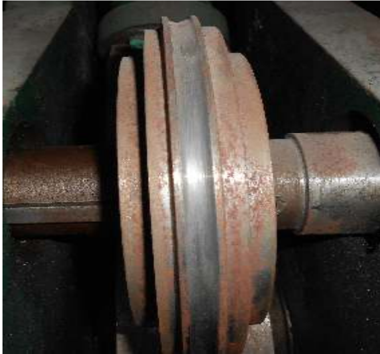
Figure 4.7 : Coining Wheel for 8 mm feedstock material
