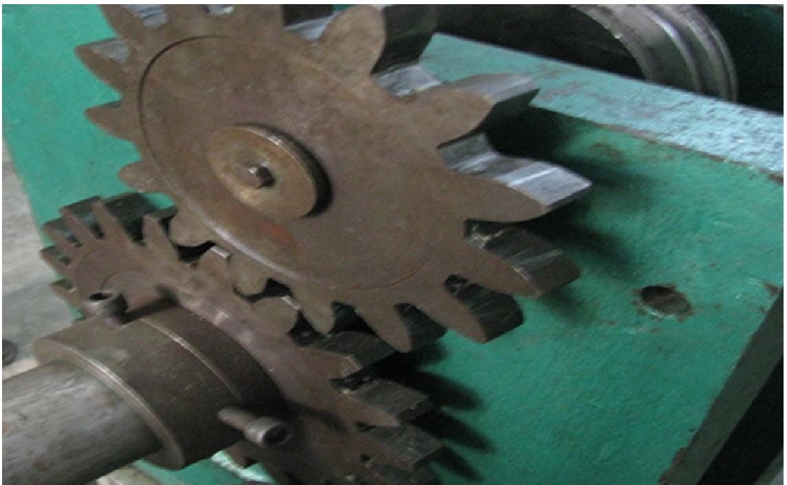
Figure 4.12: A pair of spur gear for modification of 8mm feedstock Continuous Extrusion setup
