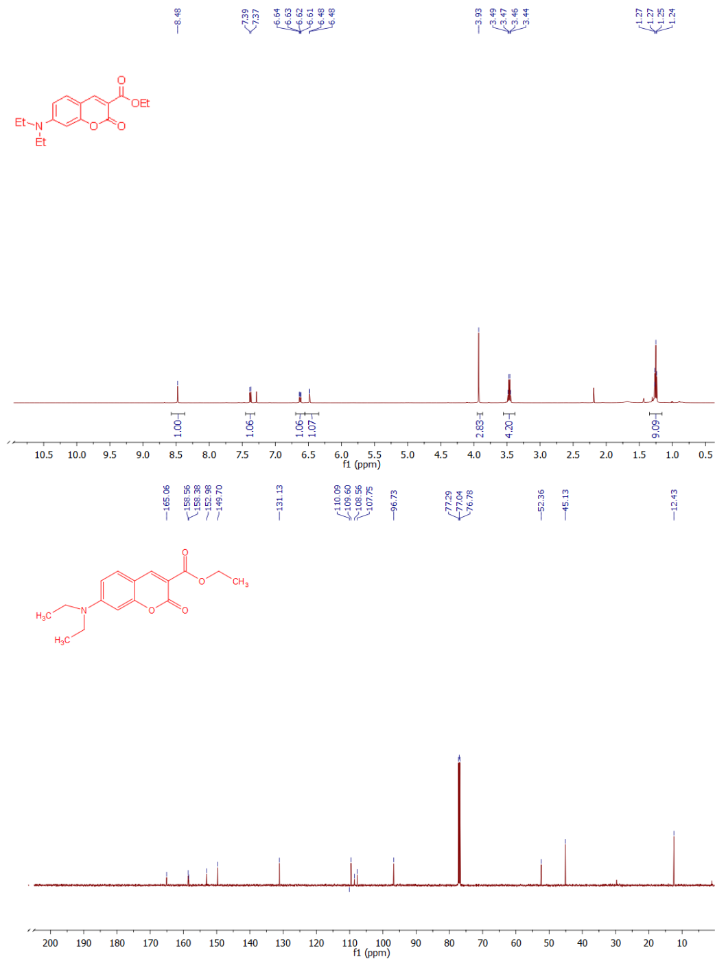
Figure 2.10: ^1\text{H} and ^{13}\text{C} NMR spectra of ethyl 7-(diethylamino)-2-oxo-2H-chromene-3-carboxylate (3e).
