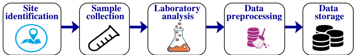
Figure 3.3: Steps involve in Lab dataset collection of the river water.
