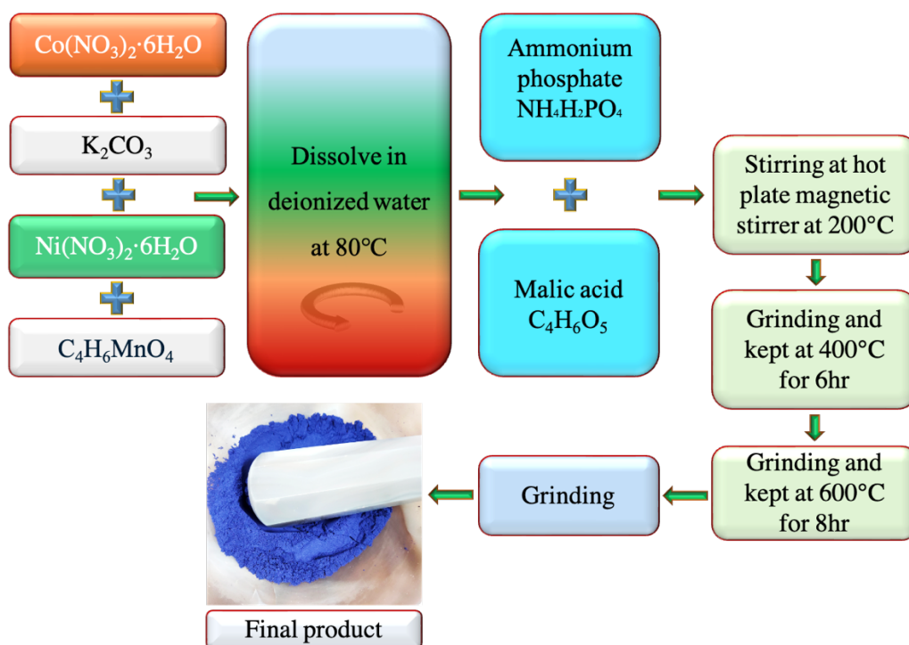
Figure 5.1: Synthesis procedure of \text{KCo}_{0.5}\text{Ni}_{0.4}\text{Mn}_{0.1}\text{PO}_4 sample
