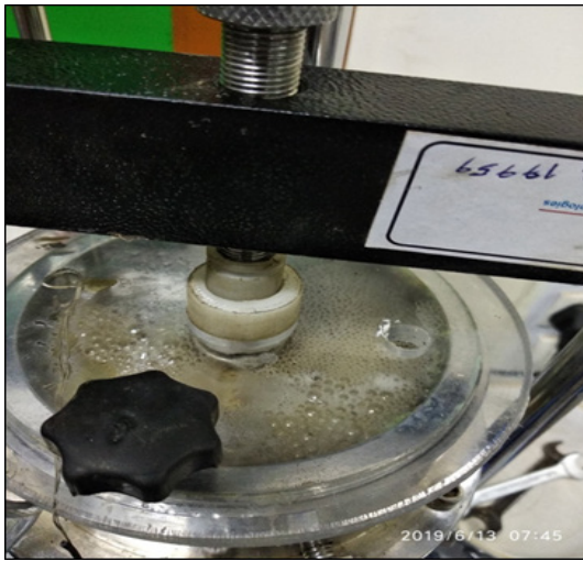
(a.) Bubble formation during the initial stage of coupled loading
