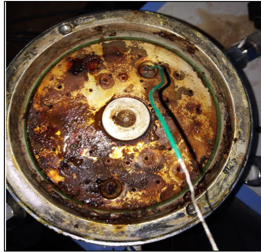
(b.) Top view of consolidation ring after completion of the test
