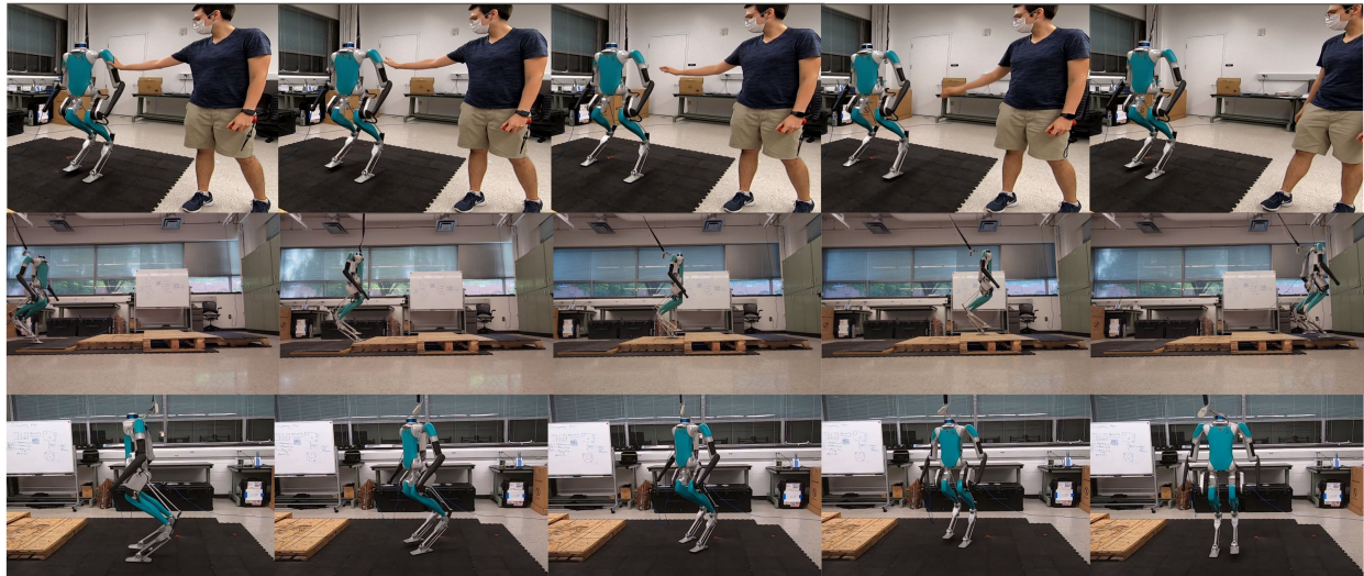
Fig. 6. Tile plots of Digit recovering from a external push (top), blind walking on terraced surface (centre), and turning in place as per command (bottom) using the learned linear policies.
