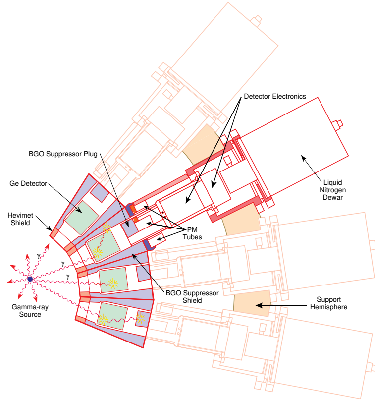
Figure 2.3 Schematic diagram of HPGe detector with Compton suppression shield. Figure taken from Ref. [1].
