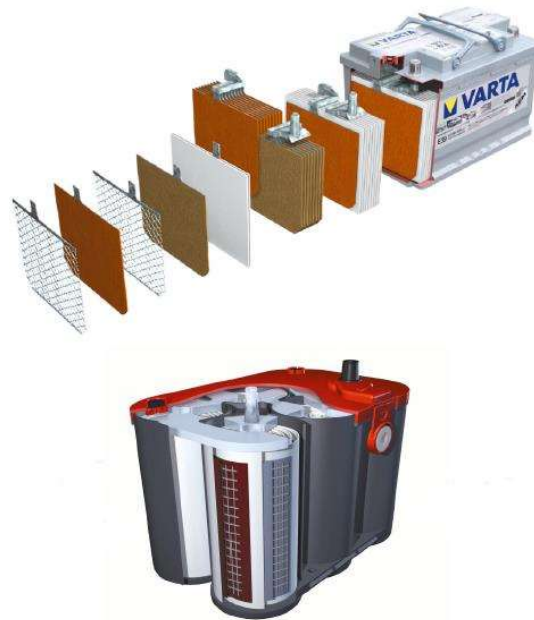
Figure 1.7 Scheme of prismatic and spiral wound construction of Lead Acid battery [25]
