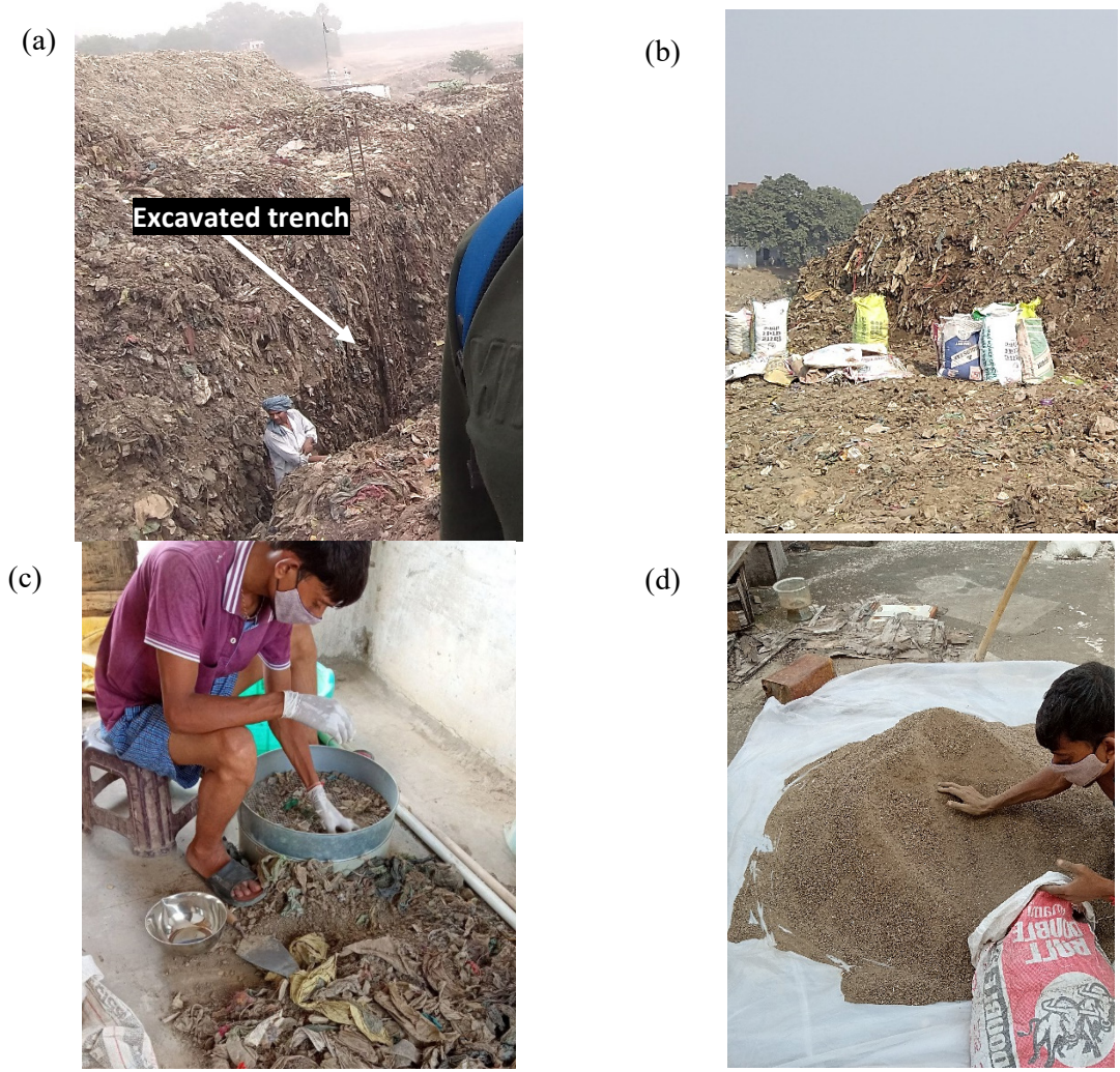
Figure 12: (a) Section of Excavated Dumpsite (b) Collection of Samples in Bags (c) Sorting Process of Legacy Waste (d) Sieved and Isolated Municipal Solid Waste Fines
