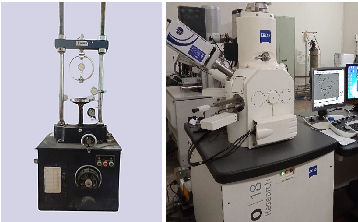
Figure 14: (a) A photograph of UCS testing machine, (b) A photograph of high-resolution scanning electron microscope (SUPRA 40, Zeiss 4.0)
